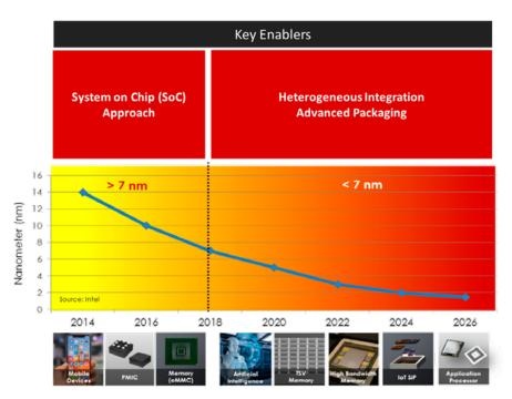
Figure 1: Packaging evolution vs. fabrication technology. SOURCE: Intel
