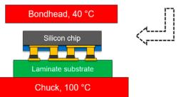
Figure 5: Fluxless TCB process.
