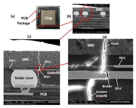
Figure 7: Failure modes of the fan-out lead-free package PCB assembly subjected to a drop test (>500 drops): a) The fan-out package PCB assembly; b) Cross section of the assembly; c) and d) Close-up of a cracked RDL; a cracked EMC; and a cracked underfill (but no crack in the solder joint).
