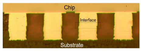
Figure 11: Chip-to-substrate as-plated copper pillar bond.
