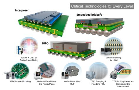
Figure 2: Packaging technologies in different HI levels.
