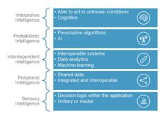
Figure 3: Quality intelligence levels: A holistic quality approach can be addressed in terms of levels of intelligence, starting with sensory intelligence, in which quality systems can make decisions within the scope of their data.
