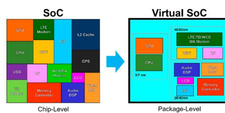
Figure 2: Splitting the SoC and reintegration.
