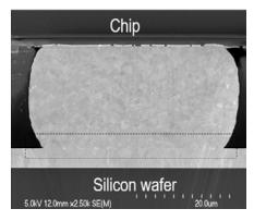
Figure 9: Chip-to-wafer as-plated copper pillar bond. The interface is highlighted with a dotted line.
