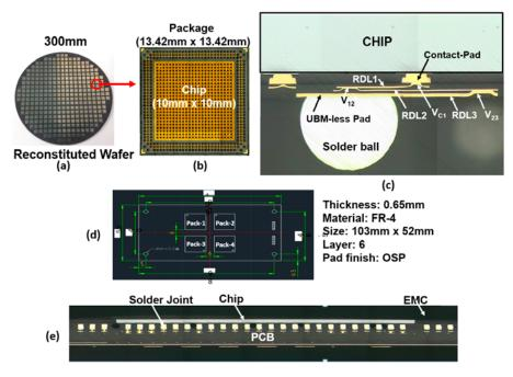
Figure 2: Fan-out package with lead-free solder joints on a PCB.
