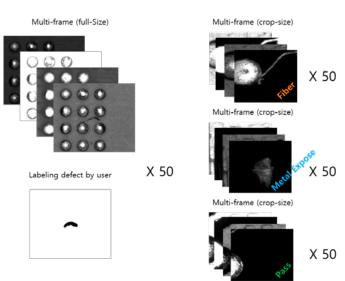
**Figure 2:** The deep-learning model training process: a) (left) segmentation; b) (right) classification.
