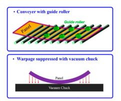
Figure 7: Physical warpage suppression methods.
