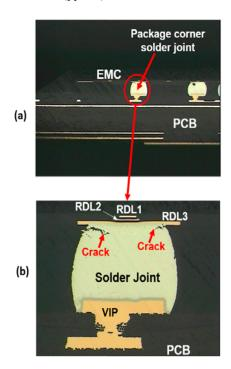
**Figure 4:** a) Failure location, and b) failure mode of the fan-out package with lead-free solder joints on a PCB subjected to thermal cycling.
