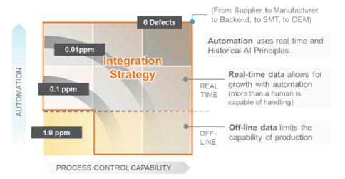
**Figure 1:** An illustration of end-to-end quality. Moving decisions from offline human decisions to real-time decisions based on data patterns enables factories to increase product quality.
