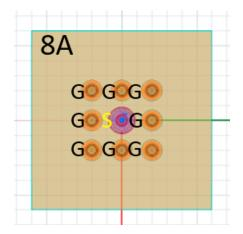
**Figure 1:** Example of an optimum signal/return pin layout.
