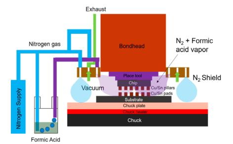
Figure 1: Schematics of a formic acid delivery system with a bond head shroud.
