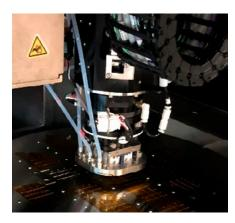
Figure 3: Shroud mounted on the bond head.
