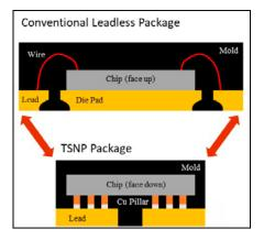
Figure 1: Package shrink-wire bond versus flip chip.
