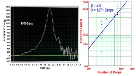
Figure 6: Drop spectrum and Weibull plot of the drop test results for the fan-out package with lead-free solder joints on a PCB with underfill.
