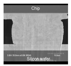
Figure 10: Chip-to-wafer fly-cut plated copper pillar bond. The interface is highlighted with a dotted line.
