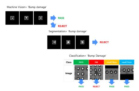
Figure 3: Deep-learning inspection progress using segmentation and classification combined algorithms.
