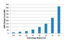
Figure 1: Design cost over technology node [1].
