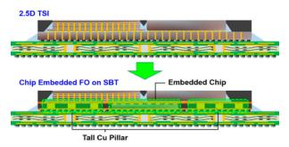
Figure 8: Chip embedded fan-out packaging.
