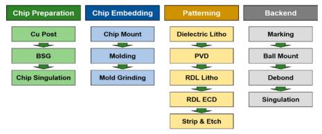
Figure 6: Chip-first face-up fan-out process flow.
