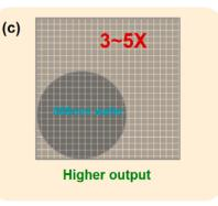
Figure 4: The geometrical benefit of panel-level packaging.
