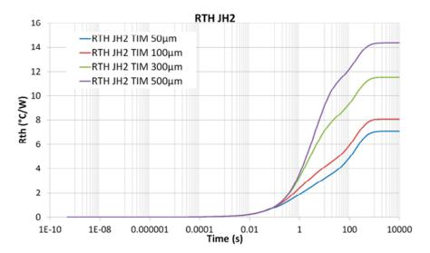
Figure 5: Impact of TIM thickness on Rth (T<sub>amb</sub> 85°C; P<sub>diss</sub> 5W).
