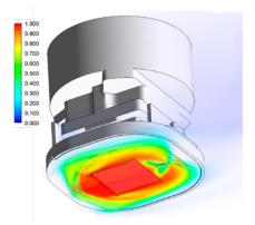
**Figure 4:** Mass fraction of FA vapor in  $N_2$  over the chip area.
