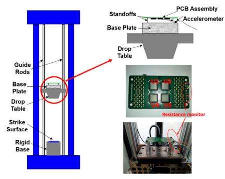
Figure 5: Drop test setup.
