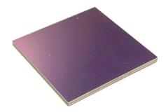
Figure 6: A 30mm die-to-die bonded assembly.
