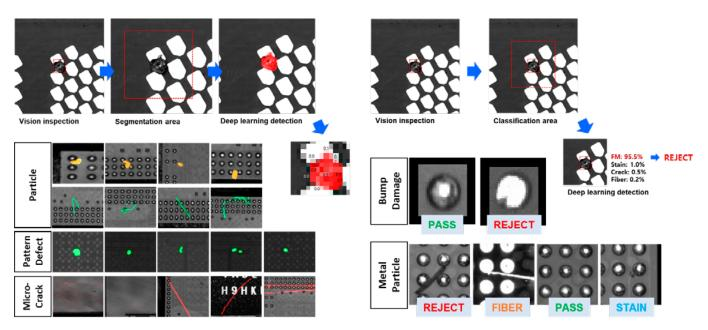
Figure 1: a) (left) The diagrams show segmentation inspection progress and results. Defect size can be measured accurately to determine a "Good" or "NG" defect based on the specification; b) (right) The diagrams show classification inspection progress and results. Different classes for each defect and multiple classes within each defect can be classified as applicable.
