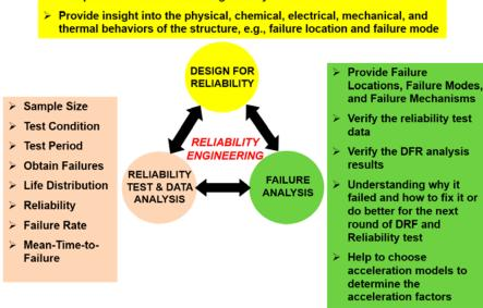
Figure 1: Reliability engineering: design for reliability, reliability testing and data analysis, and failure analysis.
