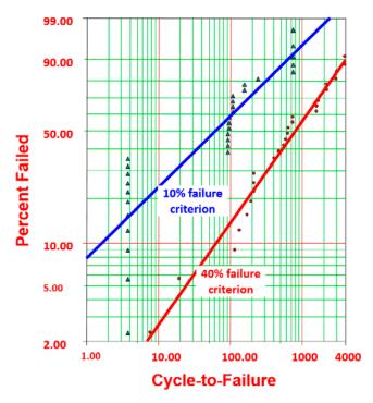
Figure 8: Weibull plots of a 208-pin PQFP with 10% and 40% resistant change failure criteria.
