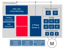
Figure 2: An EPS system diagram [2].
