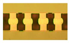
Figure 7: A fluxless TCB sample.
