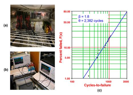
**Figure 3:** a) Thermal cycling chamber and samples; b) Data acquisition system; c) Weibull plot of the thermal cycling results for the fan-out package with lead-free solder joints on a PCB without underfill.
